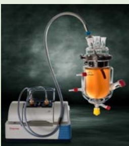
Fig.2 FTIR-spectrometer iS5 with ATR-fiber probe
