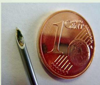
Fig.3 Needle ATR-PIR-fiber probe
