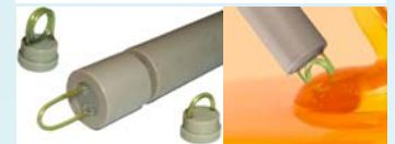
Fig. 4. Transmission spectra of different ATR-probes of 1,5m length and design of detachable single & multi-loop ATR-tips.
