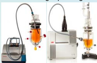
FTIR spectrometers equipped by DTGS-detectors & coupled with ATR-fiber probes by mirror-fiber couplers installed in sample chambers. Fig. 1. Fiber coupled FTIR from Thermo (iS5) and ABB
